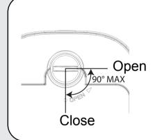
Turn the knob 90 degrees clockwise to lock the battery cover.
