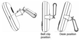
1. The belt clip/stand attaches to the back of the parent unit and clips into the locking slots on each side.
