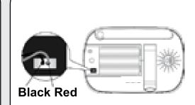
Insert the wire tab of the rechargeable battery pack into the contact slot as shown above and fit the battery pack into the compartment.
