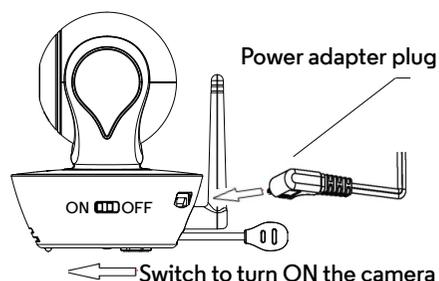
1. Insert the power adapter plug into the micro USB socket at the back of Camera unit.
